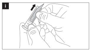
To change the blade, pull the holder all the way out of the body.
