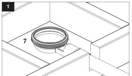
Connect the outlet section (7) securely to the waste pipe system to ensure no leaks.
