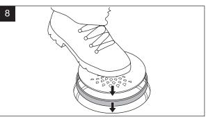
Place the clamping ring with the text up and put the grating on top of it. Press them both firmly down in to the gully until they are fully fixed.
