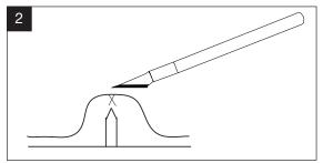
For vinyl/pvc cut a cross in the membrane so that the spike will appear.
