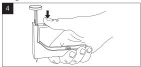
Apply slight pressure on the arm release knife holder so the blade locks in to position.
