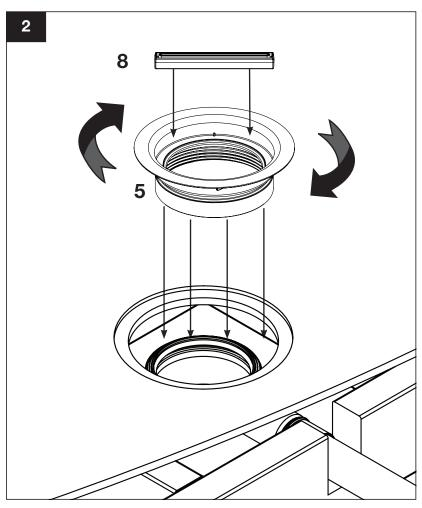
Grab the outlet section (7) with one hand and start screwing on the middle section (5). Then continue using the installation tool.
