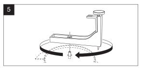
Place the arm of the knife on the spike and spin the knife 360 degrees cutting.
