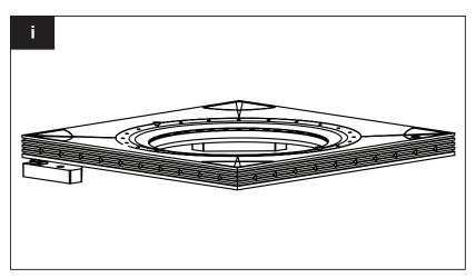
For installation in floor boards when not using a former tray use the Purus plate 130 Art.no 713 36 81 or Purus multiplate Art.no 713 36 90
