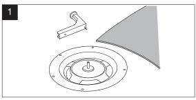
After having removed the clamping ring place the Purus knife bottom section in the clamping ring seat in the floor gully.
