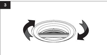
Screw down the middle section (5) firmly with the installation tool so that the middle (5) and the outlet sections (7) are fully fixed together.
