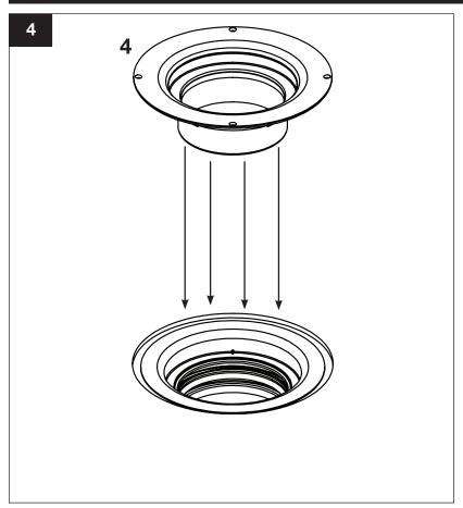
Push the top section (4) firmly inside the middle section (5) until they click together. The gasket (6) should not be visible when the top section (4) is installed correctly.
